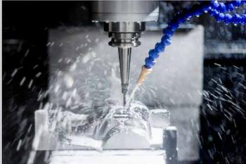
**Milling** - is a very universal fabrication method with great accuracy and tolerances. Milling is suitable for a variety of materials and is also very quick. The ability to manufacture a wide range of complex parts is a great advantage.
