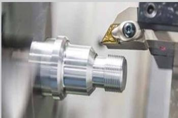
**Turning** - while the two are often called just CNC machining, turning and milling have distinct differences. Turning is pretty much the opposite of milling. This means that instead of the cutting tool, the workpiece is rotating. For example, CNC turning is commonly used for producing shafts.
