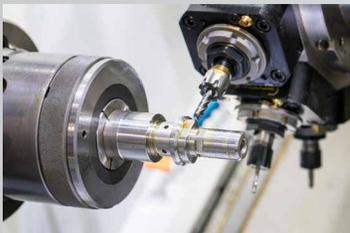
**Drilling** - While milling equipment can also produce holes, drills are meant for only that job. The difference? While milling tools use cutting edges around the cutting head's periphery, drills use the tip of the tool to produce a hole. CNC drilling machines are commonly used to automate this job, provide better accuracy and a more cost-effective solution.
